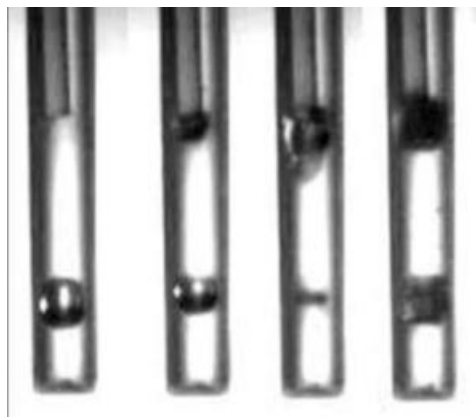
Fig. 4. An air inclusion being compressed when the bubble grows and expands—settings: 25 mJ, 20 Hz.
