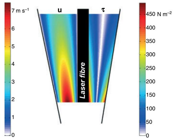
**Figure 4** Average velocity profile (left) and shear stress distribution (right) between two concentric cylinders of which the outer cylinder represents the tapered root canal wall. The average velocity at the laser fibre tip is set at  $5 \text{ m s}^{-1}$ . The region below the laser fibre tip is intentionally left blank, as details of the streaming pattern in the apical part are missing and are part of a future study.
