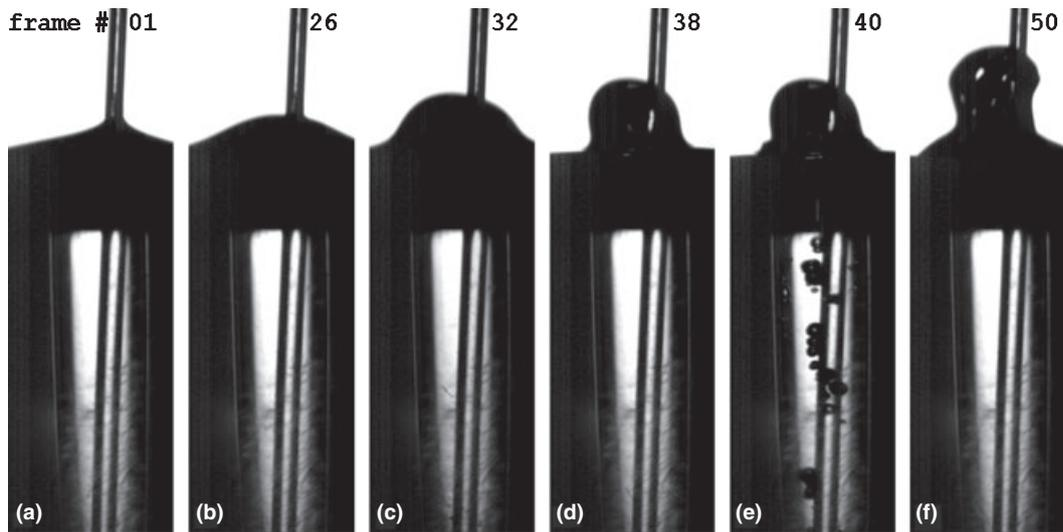
**Figure 3** (Video clip S3) Pinch-off at the free surface at the coronal part of the glass root canal model. Secondary cavitation bubbles are formed (in *e*) upon passage of a shockwave generated by the vapor bubble inertial collapse at the laser fiber tip. The frame rate is 14,000 frames/second.
